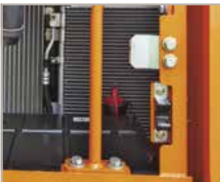
Battery cut-off switch
