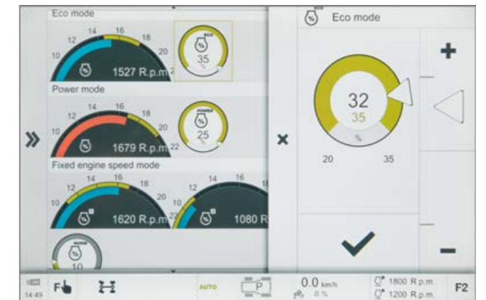
Engine droop setting for "Eco" and "Power", and the engine speed memory
