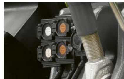
When a front linkage is installed, up to four hydraulic connections and one free-flow return line are available at the front. Ideal for a front-mounted seed hopper or dozer blade.
