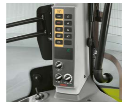
The PTO speed and electronic rear linkage control system can be adjusted on the B-pillar.
