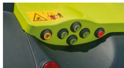
External controls for the rear linkage, PTO and one freely selectable spool valve (CEBIS only).
